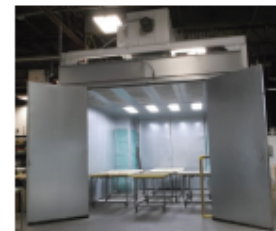
Batch Cure Chamber Interior
